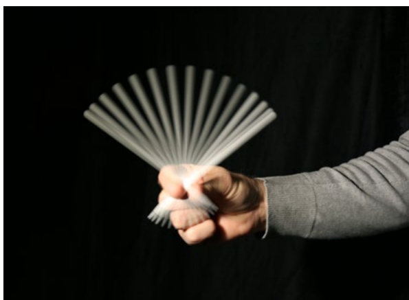
Figure 2: Illustration of stroboscopic effect. Photo: J.Rydeman
